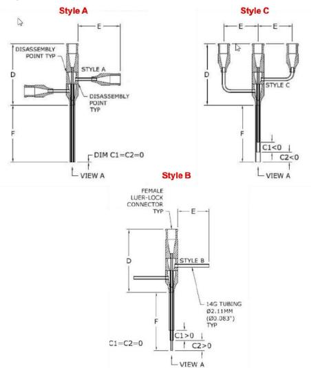
Dim D is approximately 30mm and is not adjustable Disassembly for cleaning at point "POS"
