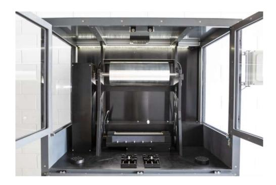
E-Fiber EF500 version is a scale-up of the traditional electrospinning technique, capable of manufacturing batches of large format nanomatrix (up to 50 x 80 cm) or roll-to-roll reels, including dual high voltage power supply, touch screen console for the control of all the parameters (spinneret and collector rotating speed, spinneret-collector distance, applied voltage), and insulated enclosure.
