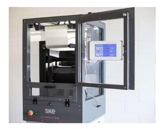
E-Fiber EF500 Desktop version is a scale-up of the traditional electrospinning technique, capable of manufacturing batches of large format nanomatrix (up to 60 x 30 cm) or roll-to-roll reels, including dual high voltage power supply, touch screen console for the control of all the parameters (spinneret and collector rotating speed, spinneret-collector distance, applied voltage), and insulated enclosure.
